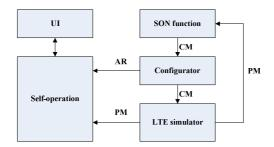
**Fig. 4.** Architecture of self-operation demonstrator for learning operation experiences, where AR = action request, CM = configuration management data, PM = performance management data, and UI = user interface.
