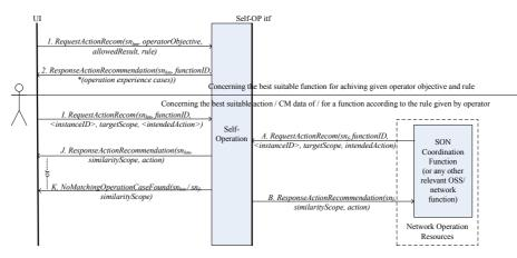
Fig. 1. The architecture of defining and applying similarity measures based on stored operation experience cases.
