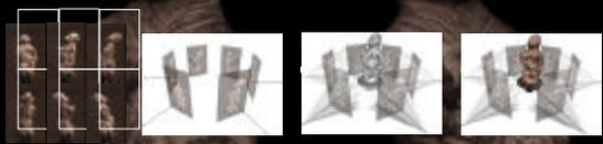
Image acquisition    Camera calibration    3D reconstruction    Texture map creation
