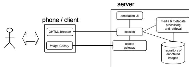
**Fig 3.** The main components of the *MMM* system.
