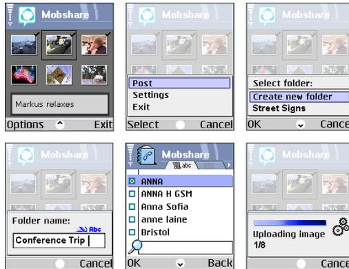
**Fig 4.** . The picture uploading and sharing process where a) the images are selected, b) the upload is initiated, c) a new folder created, d) named, e) the people selected, and f) finally the images are uploaded.
